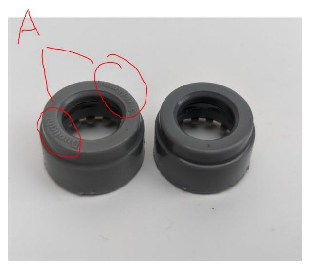
As shown in the image above the new fittings made from POK are shown on the left and the older POM fittings are shown to the right. This change to the injection moulded tooling was made so the parts made from the different polymers were easily distinguishable.
