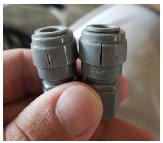
As this outer ring that pushes over the fitting is under some tension/stress this part was more susceptible to the chemical attack.
